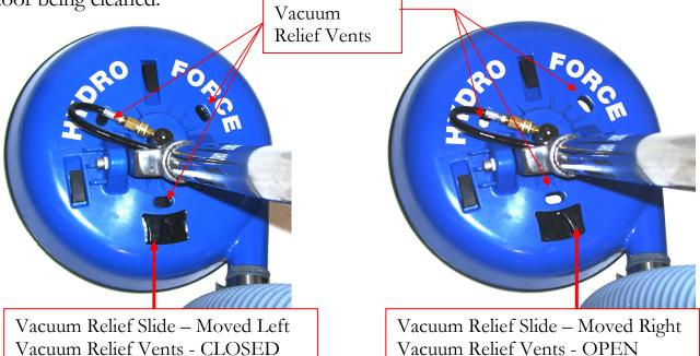
Using the SX-15 with extractors with higher air flow will generally require the vacuum relief vents to be opened more.
