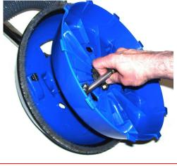
Separate the Outer & Inner Shells
